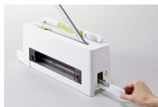
Pulling out the old blade
