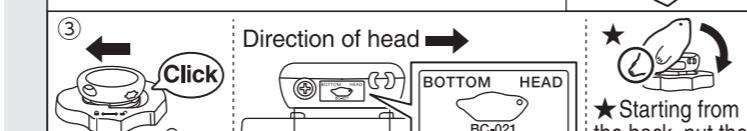
③ Refasten the screw. Return the blade base to the cutter and lock it. Refer to the illustration on the blade base to ensure the silicone cover is facing in the correct direction. Starting from the back, put the silicone cover back on the cutter.
